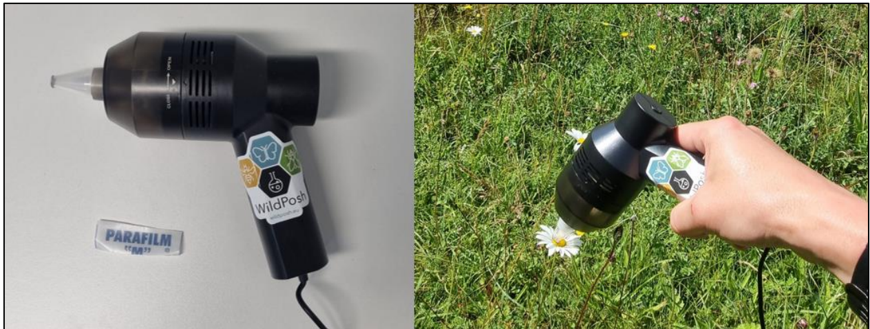
Figure 5: The electronic pollen sampler (“E-PoSa”), based on a USB powered portable vacuum cleaner (left) and the device in action (right).
