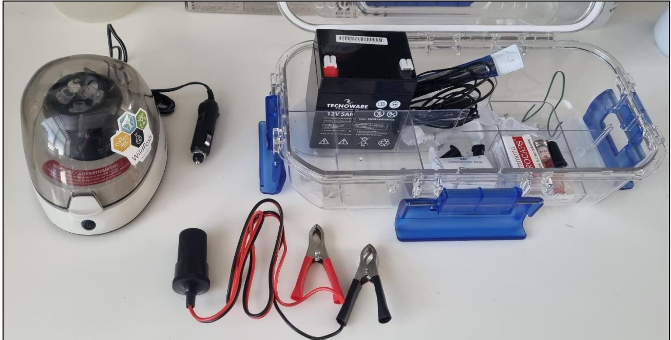
Figure 6: Field centrifuge kit. A tabletop centrifuge with a car plug, a cable with car socket that can be attached to a battery. A carrying case with a 12V battery and supplies.
