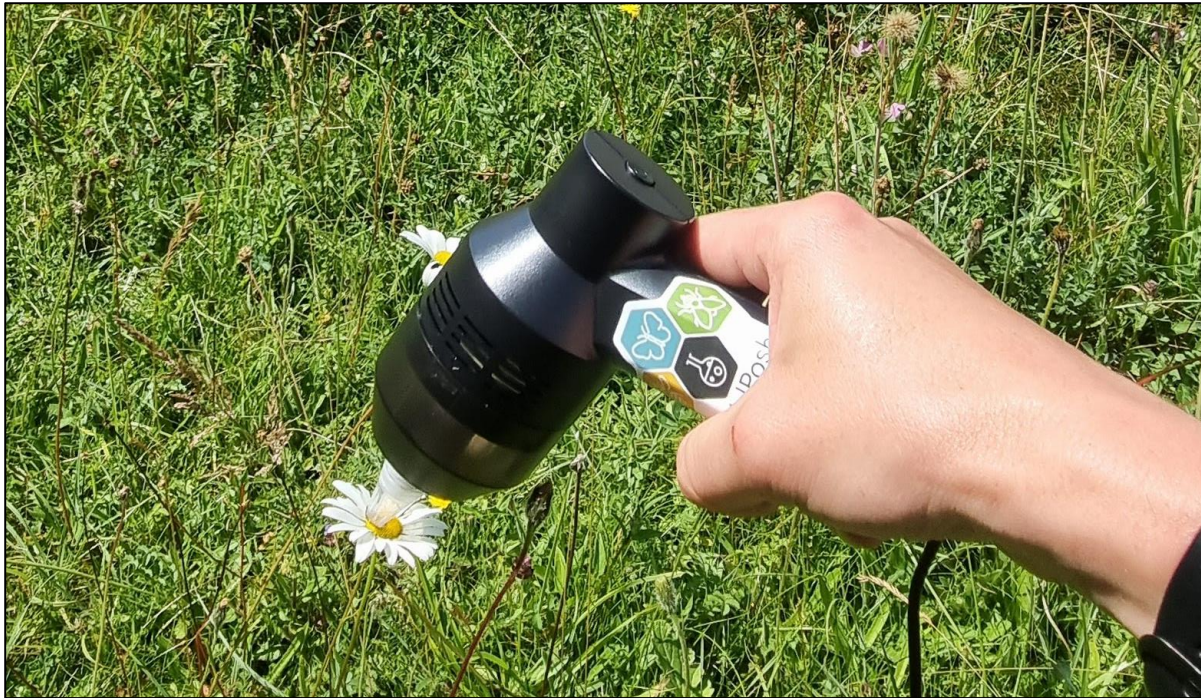
Figure 3: Extracting pollen using the electronic pollen sampler in the field. Gloves should be used when collecting actual pollen samples.
